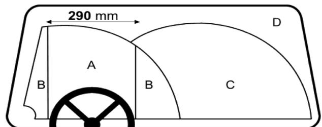
Zone A Damage up to 10mm | Zone C Damage up to 25mm
